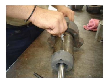
step 6 Slide the choke indicator (13) onto the stem (10) with the "zero" end facing away from the choke bonnet (2) – do not tighten yet.
