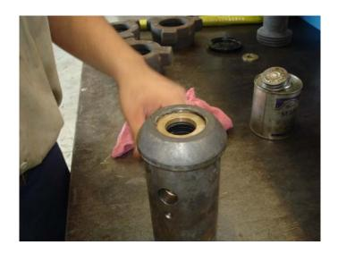
Install snap ring (8). Use snap-ring pliers to install
