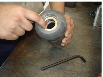
**Note:** Install packing set (9) with thick back-up ring against the stem guide (6). The thin portion of the packing set will be facing the opening of the 1502 opening.
