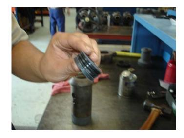
**Note:** This image is a closer look at the packing set arranged in the order that it should be installed.
