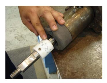
step 7 Attach the handwheel(14), washer (15), and hex nut(18) onto the stem (10).
