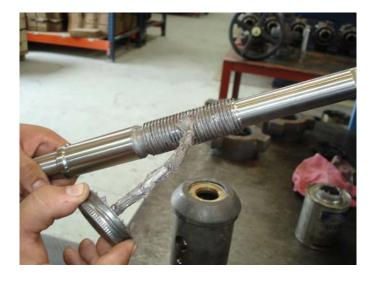
step 4 Apply anti-seize to the threads of the stem (10). Insert the end of the steam, opposite the carbide, into the packing and carefully push straight in until the threads of the stem meet and engage the threads of the bonnet. Turn the stem clockwise until the raised ring below the sealing area of the stem bumps against the packing retainer (7).
