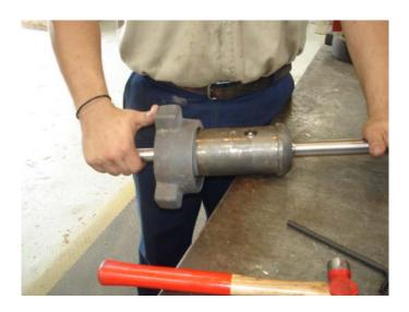
Installing thumb screw (12).
