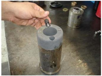
step 3 Apply anti-seize in the packing gland of the bonnet body (2) and install the following in order:
