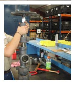
**step 9** Line up the "zero" calibration of the indicator **(13)** with the indicator groove on the end of the bonnet extension **(6)** and tighten the setscrew in the indicator **(13)**. Note-This step is required whenever the bonnet assembly **(2)** has been disengaged from the tee assembly **(1)**.
