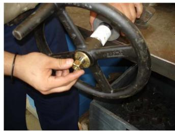
step 8 Mount the bonnet assembly to the choke tee assembly with a good choke seat (21) and make up the union properly. Crank the hand wheel (14) clockwise to the full closed position, until the stem bottoms out firmly into the choke seat.
